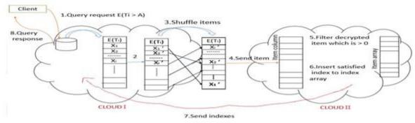
Fig. 4. Query protocols(Each step is marked 1,2,3..
